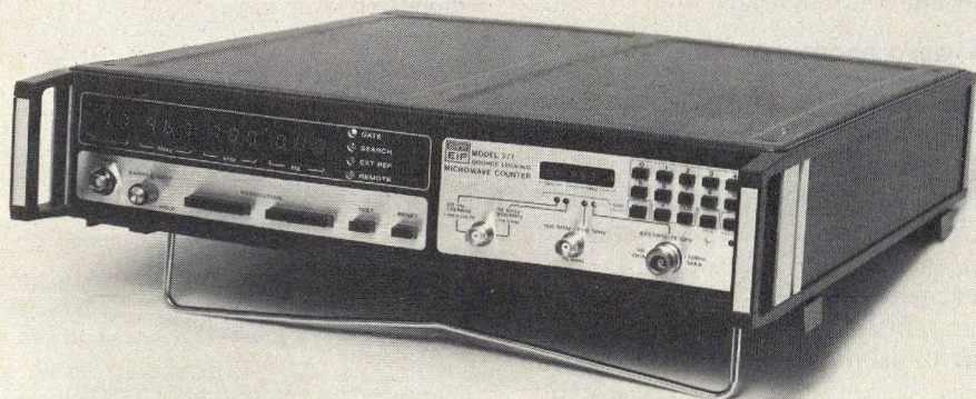
1. Source locking capability is added to a frequency counter without any increase in size. Cost is about $1,000 more than the counter alone.
